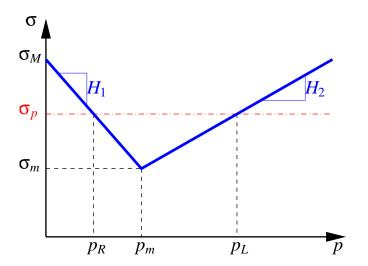
peak stress:  $\sigma_M$ , minimal stress:  $\sigma_m$ , plateau stress  $\sigma_p$ , Lüders strain  $p_L$ , hardening moduli  $H_1 < 0, H_2 > 0$ .
