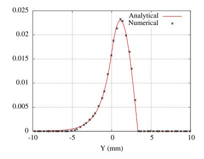
Analytical and finite element plastic strain rate profiles  $\dot{p}$
