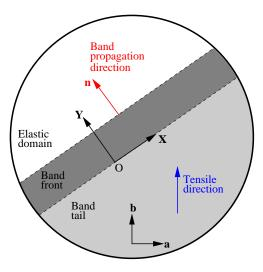
Homogeneous tensile stress state. The strain localization band in 2D (Rice's criterion) is inclined at  $54.7^{\circ}$  from the tensile axis
